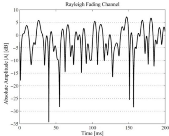
Fast fade of radio signal vs. time
